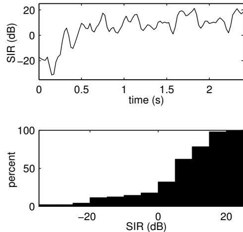
Fig. 1. Local SIR for  $\hat{s}_1$  estimated by FICA and TI Filt decomposition in the  $2 \times 2$  convolutive mixture. Hanning windows of length 100 ms and overlapping 75 ms are used. The SIR is plotted against time in the upper plot and summarized in a cumulative histogram in the lower plot.
